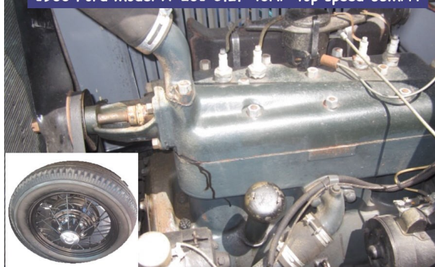
1930 Ford Model A~201 C.I.~40HP~top speed 65MPH
